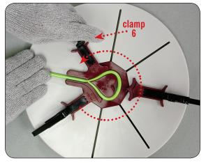
After the first clamp is in place, move the pen tube around the entire shape mold as shown and slowly close clamp number six.
