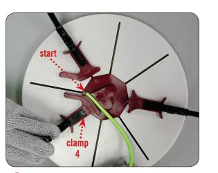
With a sufficiently heated pen tube, place the heated end of the tube at the start position shown above and slowly close clamp number four.
