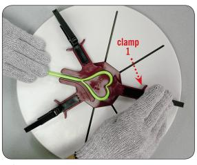
Finally, slowly close clamp number one. Wait until cool and remove by using the grip/pry tool.
