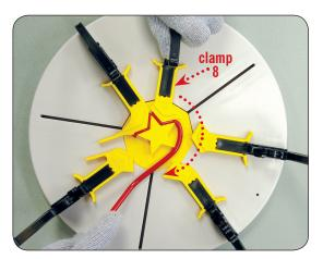
2. After the first clamp is in place, move the pen tube around the entire shape mold as shown and slowly close clamp number eight.
