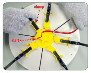
With a sufficiently heated pen tube, place the heated end of the tube at the start position shown above and close clamp number seven.
