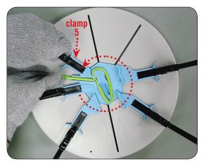
2. After the first clamp is in place, move the pen tube around the entire shape mold as shown and slowly close clamp number five.
