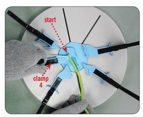
1. With a sufficiently heated pen tube, place the heated end of the tube at the start position shown above and close clamp number four.
