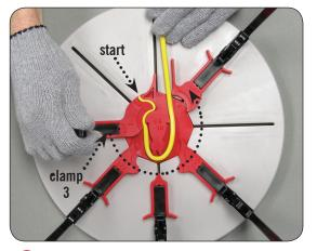
With a sufficiently heated pen tube, place the heated end of the tube at the start position shown above and close clamp number three. Next, move the pen tube around the entire shape mold as shown above.
