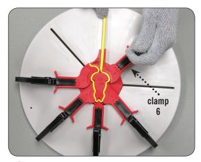
6. Finally, slowly close clamp number six. Wait until cool and then remove by using the grip/pry tool.
