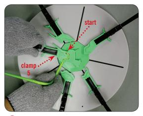
With a sufficiently heated pen tube, place the heated end of the tube at the start position shown above and slowly close clamp number five.
