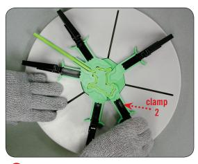
6 Finally, slowly close clamp number two. Wait until cool and then remove by using the grip/pry tool.
