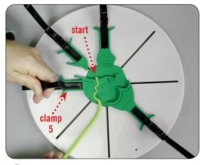
With a sufficiently heated pen tube, place the heated end of the tube at the start position shown above and slowly close clamp number five.
