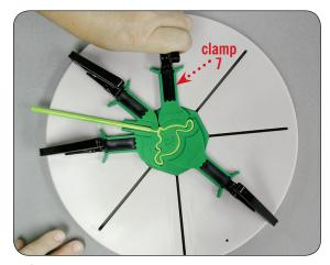
Finally, slowly close clamp number seven. Wait 4. until cool and then remove by using the grip/pry tool.
