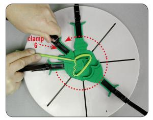
2. After the first clamp is in place, move the pen tube around the entire shape mold as shown and slowly close clamp number six.
