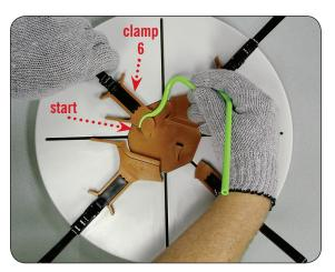
1. With a sufficiently heated pen tube, place the heated end of the tube at the start position shown above and slowly close clamp number six.
