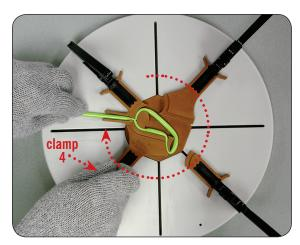
2. After the first clamp is in place, move the pen tube around the entire shape mold as shown and slowly close clamp number four.
