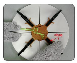
Finally, slowly close clamp number two. Wait until cool and then remove by using the grip/pry tool.
