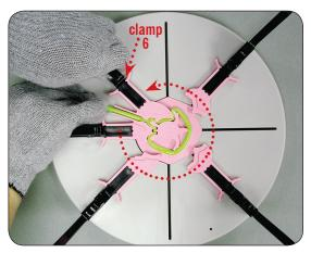
2. After the first clamp is in place, move the pen tube around the entire shape mold as shown and slowly close clamp number six.
