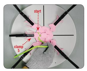
1) With a sufficiently heated pen tube, place the heated end of the tube at the start position shown above and close clamp number five.
