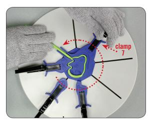
2. After the first clamp is in place, move the pen tube around the entire shape mold as shown then slowly close clamp number seven.
