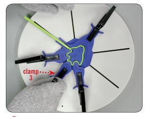
4. Finally, slowly close clamp number three. Wait until cool and then remove by using the grip/pry tool.
