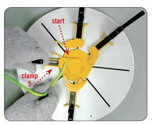
1. With a sufficiently heated pen tube, place the heated end of the tube at the start position shown above and slowly close clamp number five.
