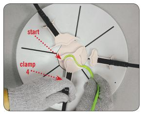
1. With a sufficiently heated pen tube, place the heated end of the tube at the start position shown above and slowly close clamp number four.
