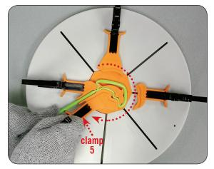
After the first clamp is in place, move the pen tube around the entire shape mold as shown and slowly close clamp number five.
