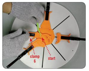
With a sufficiently heated pen tube, place the heated end of the tube at the start position shown above and slowly close clamp number six.
