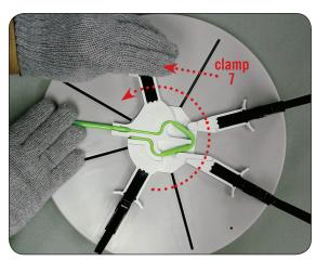
2. After the first clamp is in place, move the pen tube around the entire shape mold as shown and slowly close clamp number seven.
