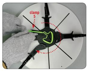
After the first clamp is in place, move the pen tube around the entire shape mold as shown and slowly close clamp number five.
