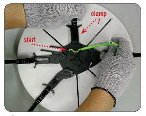
With a sufficiently heated pen tube, place the heated end of the tube at the start position shown above and slowly close clamp number seven.
