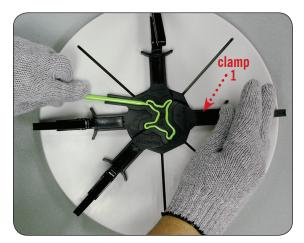
Finally, slowly close clamp number one. Wait until cool and then remove by using the grip/pry tool.
