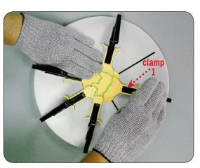
Finally, slowly close clamp number one. Wait until cool and then remove by using the grip/pry tool.
