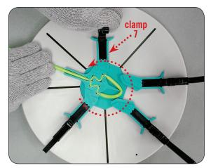
2. After the first clamp is in place, move the pen tube around the entire shape mold as shown and slowly close clamp number seven.
