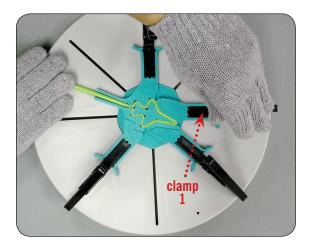
Finally, slowly close clamp number one. Wait until cool and then remove by using the grip/pry tool.
